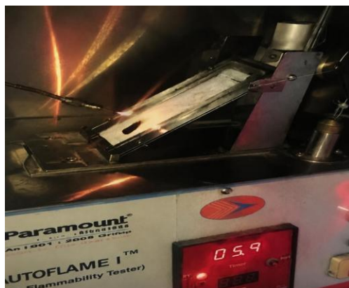
Fig. 3: Burning behaviour of CF-MC(T 2 ) cotton fabric sample in auto flammability test.
