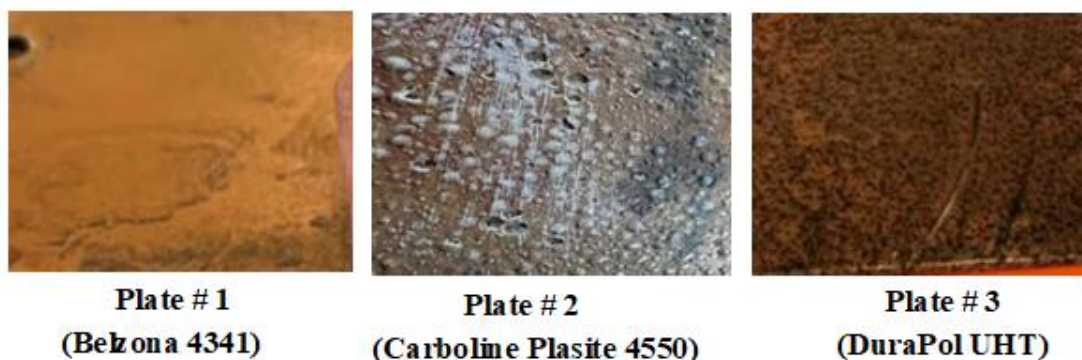
Fig. 1 Visual Test after immersion test in 98% Sulphuric acid
