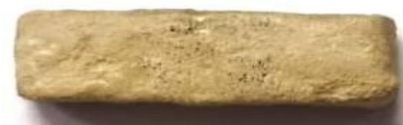
Fig.2: ZrO_2 + SiO_2 Composite powder coated on Mild Steel surface
