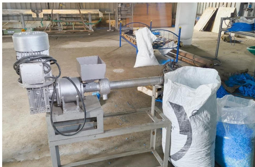
Figure 3: Hardware Prototype of the Plastic Crushing Machine
